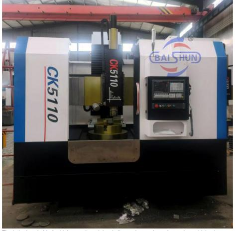
The lathe is suitable for high-speed steel, hard alloy and ceramic cutting tool, machining inner and outer cylindrical surface, inner and outer conical surface, groove and plane of ferrous metals, nonferrous metals and some non-metallic parts. It can meet different quantity production requirements with high efficiency, stable and reliable precision.
